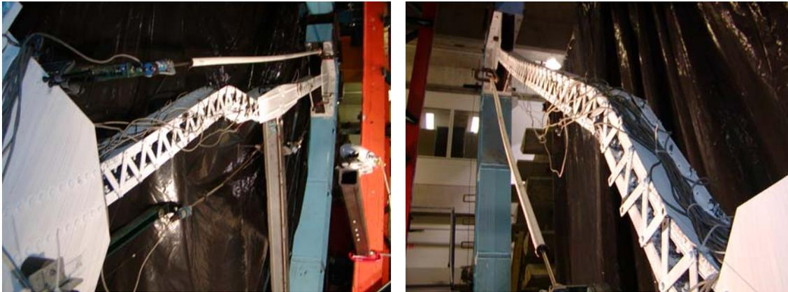
**Figure 12 - Global buckled shape of various specimens<sup>38</sup>**
